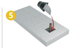
Soffit is drilled to let ducts/pipes pass through the slab.
